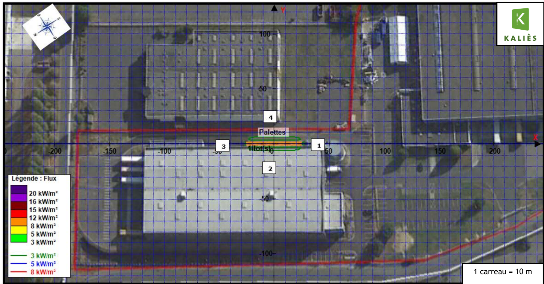
Figure 8. Incendie stockage de palettes
